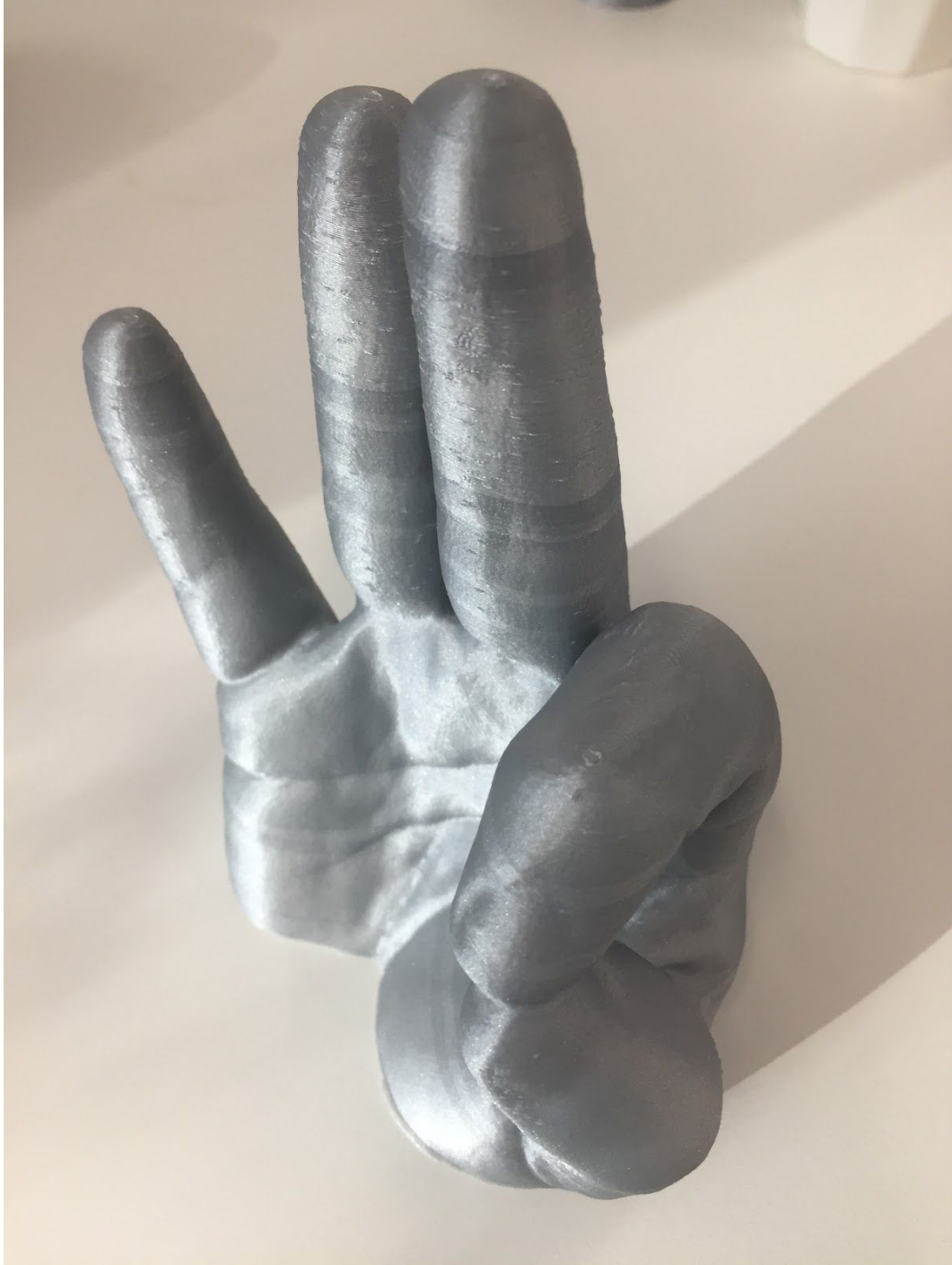
Figure [x]: Larger test print from the first final implementation in CuraEngine. Note the smoothed surfaces on top of the fingers.
